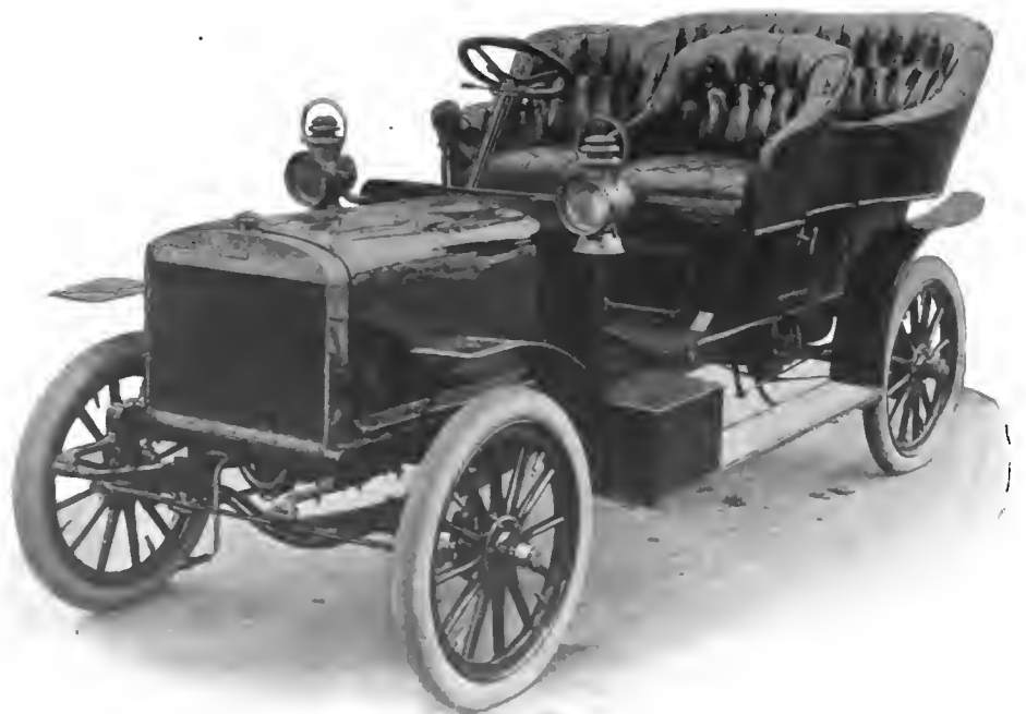
SUNSET 20-HORSEPOWER TOURING CAR DRIVEN BY FOUR-CYLINDER, TWO-CYCLE ENGINE.
